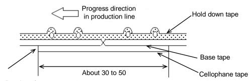
No lifting for the direction of progressing
